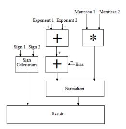
Fig. 2 Floating point multiplier
